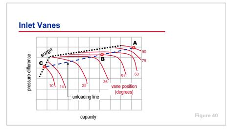
These curves represent the performance of a typical centrifugal compressor over a range of inlet vane positions. The pressure difference between the compressor inlet (evaporator) and outlet (condenser) is on the vertical axis and compressor capacity is on the horizontal axis. The surge region represents the conditions that cause unstable compressor operation.
